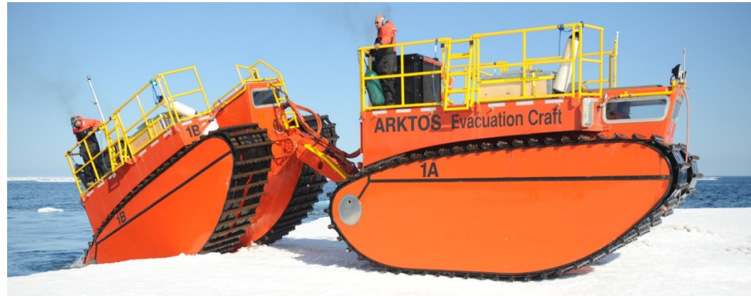
An ARKTOS Evacuation and Service Craft (spare parts shop front, 6 technicians back) climbing from deep water up a 1m+ vertical wall of ice onto an ice floe
