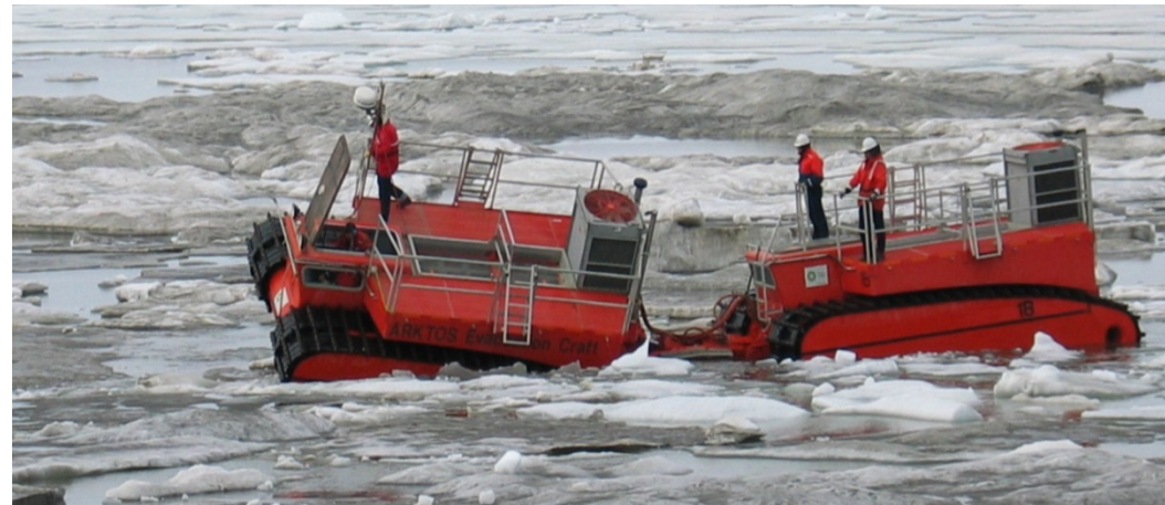
An ARKTOS Evacuation Craft (USCG approved for 52 people) operating in mixed ice and water conditions
